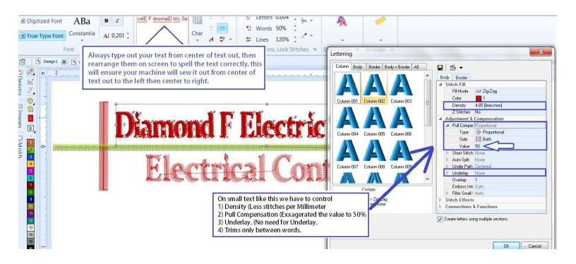
Also I set my TRIMS to WORDS. Setting trims between each letter slows the machine to a longer run time (More trims more minutes sewing) and it prevents the thread from dropping out of the needle when sewing each letter. You cannot see the connection of the stitches from letter to letter, since the machine connects the letters at the closest point.
